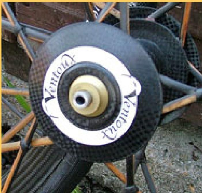
swiss 240 hubs (exactly the same as fitted to the standards) and the whoop de doos which have the dt up front, but a tune mag 160 at the rear. problem? well the dt hubs have an interchangeable freehub to suit your preference in cassettes. tune, however, offers shimano or campag, the choice being made at purchase. since i wasn't the one making the choice, the test wheel came with a shimano hub and campagnolo cassettes do not fit shimano splines.
